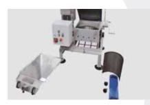
Due to the Quick snap fasteners used on the GSL series machines, the machines can be opened for cleaning and maintenance quickly without the need for special tools.
