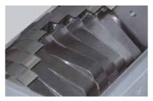
Staggered rotor blades create an individual blade cut thus increasing the cutting torque. All of the machines in this series are therefore suitable for grinding more solid materials and thicker walled sprues.
