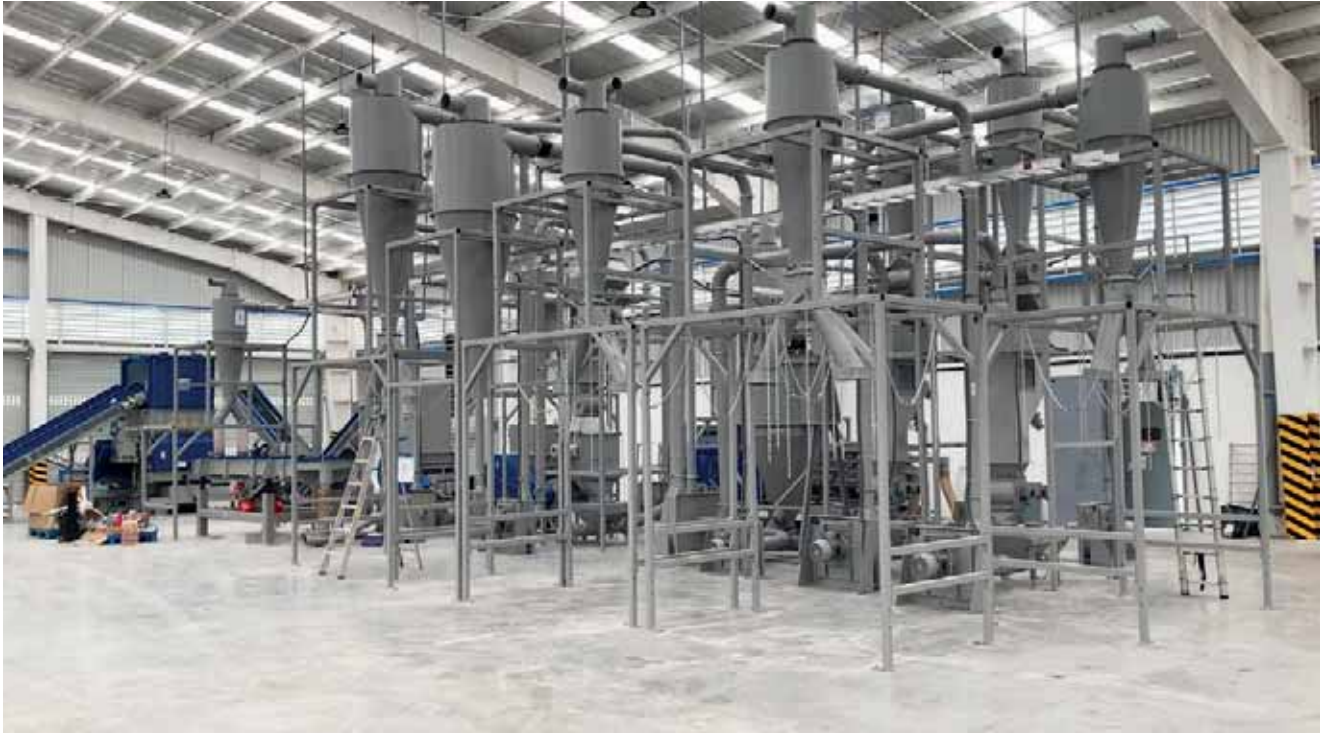
Separation and bagging station of a tire recycling line
